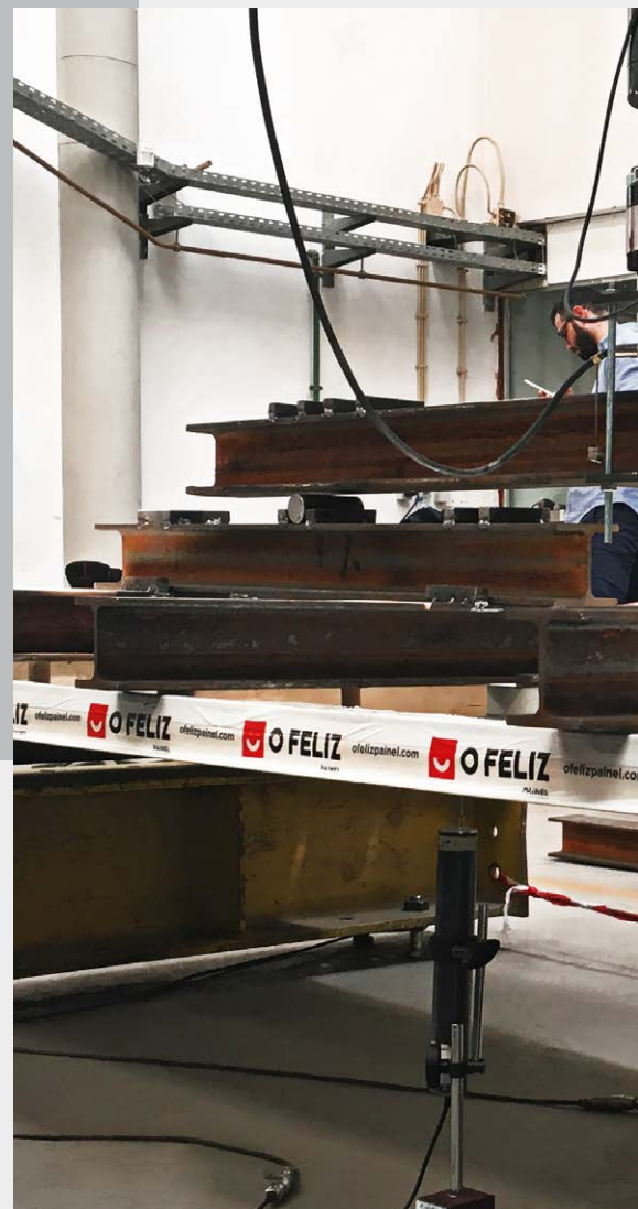
Full panel bending test
